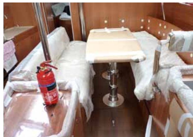
▲ Above: cardboard, pipe lagging and bubblewrap are used to protect edges and surfaces from wear
